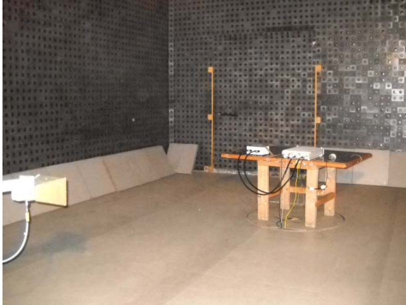
Photograph No.5 Radiated emissions measurement setup in the anechoic chamber in 1-18 GHz range
