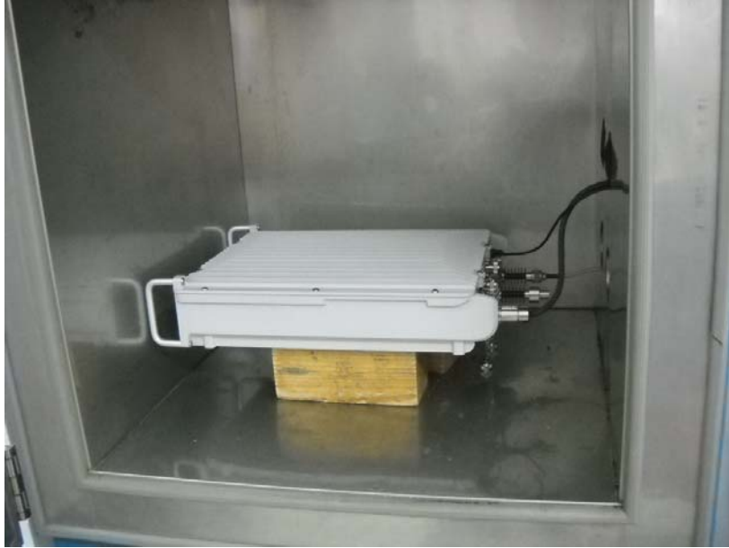
Photograph No.7 Frequency stability measurement setup
