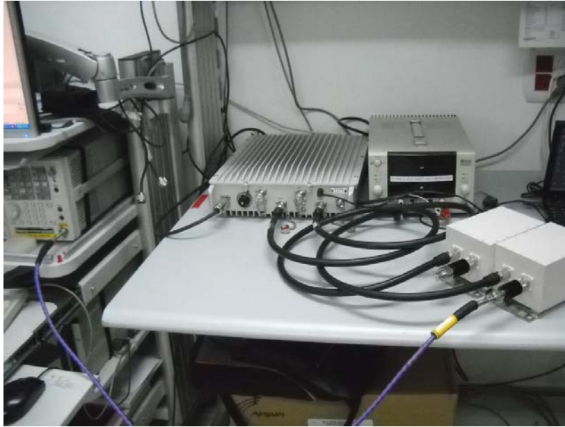
Photograph No.2 Occupied bandwidth measurement setup
