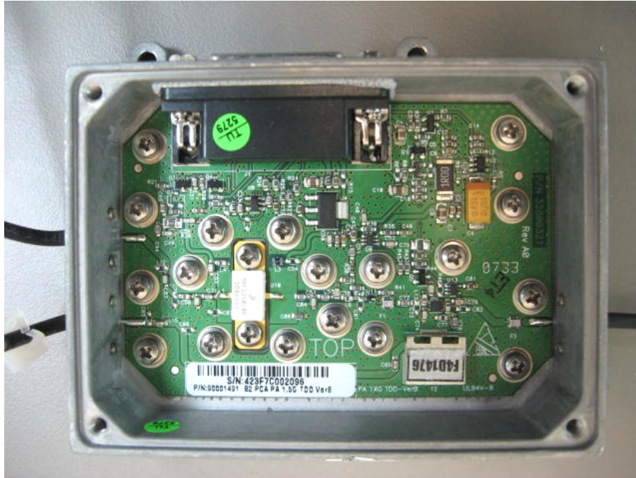
Photograph No.13 Power amplifier (PA) internal view
