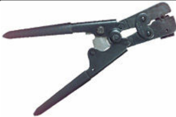
Figure 21 - Contact crimp tool
