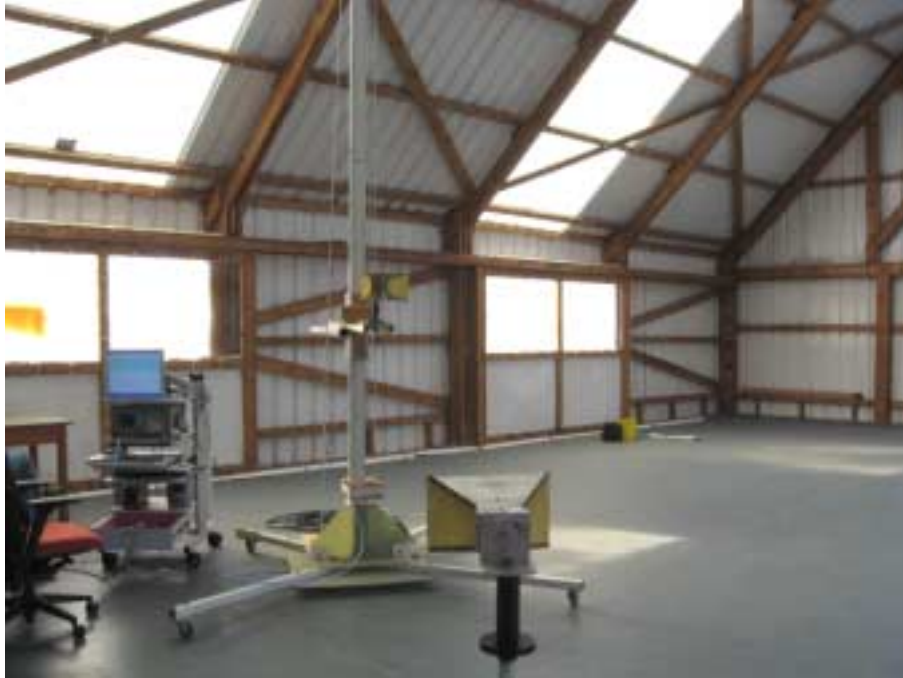
Photograph No.6 Setup of substitution ERP measurements of spurious in the anechoic chamber
