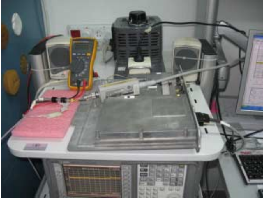
Photograph No.2 Occupied bandwidth and conducted spurious emissions measurement setup
