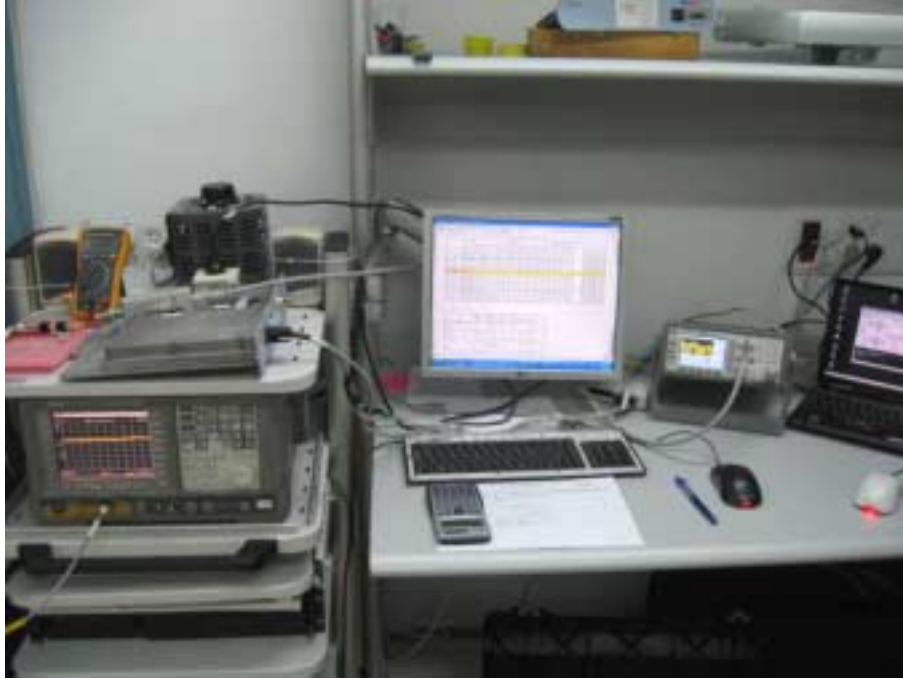
Photograph No.1 Peak output power measurement setup
