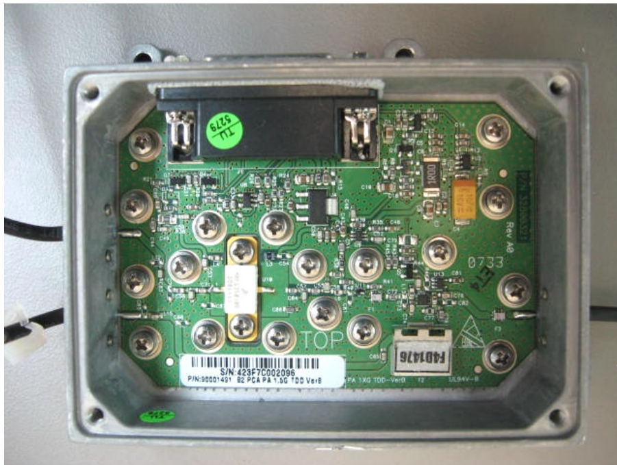
Photograph No.13 Power amplifier (PA) internal view
