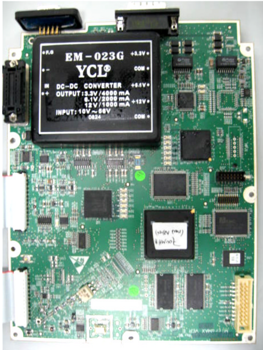
Photograph No.11 Digital interface PCB front view
