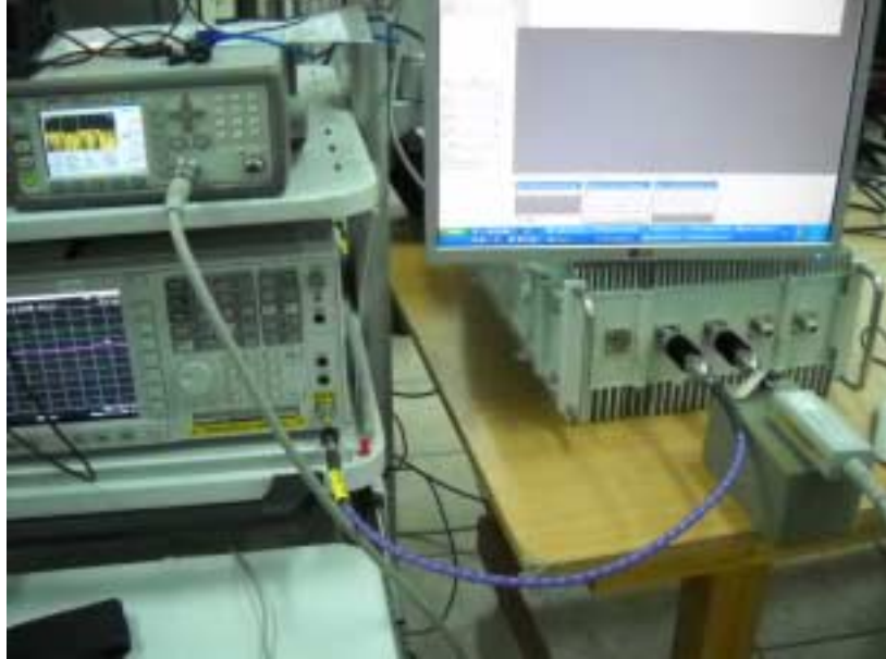
Photograph No.2 Occupied bandwidth, emission mask, conducted spurious emissions (single) measurement setup
