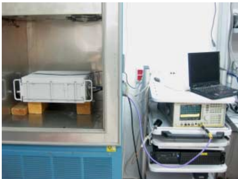
Photograph No.7 Frequency stability measurement setup
