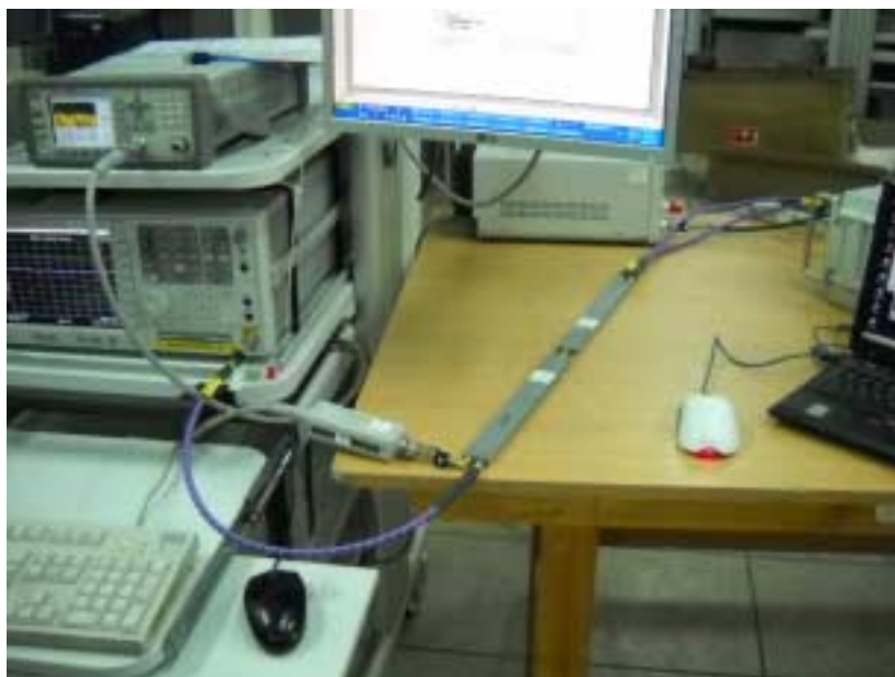
Photograph No.3 Conducted spurious emissions (combined) measurement setup
