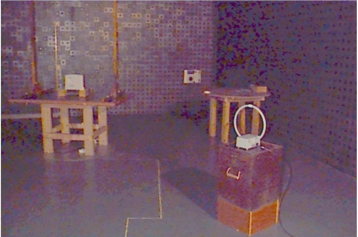
Photograph No. 4.8.1 Radiated emission measurement test setup
