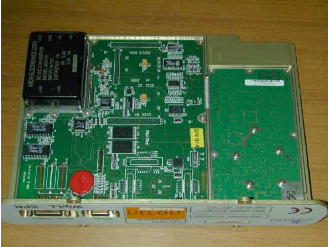
FCC ID:PIDMARCONI; SPR-2.4 inside view without covers
