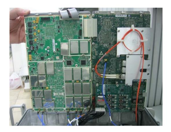
Photograph No.4 "Air4G 0707 FDD LTE" base station internal view
