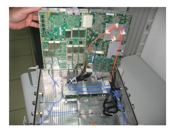
Photograph No.3 "Air4G 0707 FDD LTE" base station internal view
