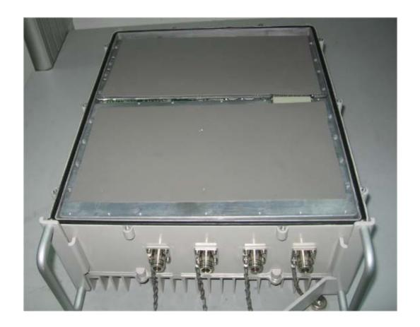
Photograph No.2 "Air4G 0707 FDD LTE" base station internal view
