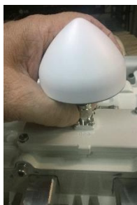
Figure 6: Attaching GPS antenna to unit
