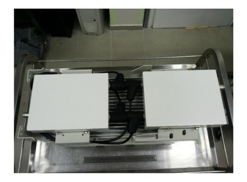
Photograph No.4 "AirHarmony 4000 866 MHz (B26)" base station side view
