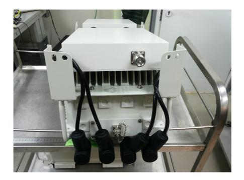
Photograph No.2 "AirHarmony 4000 866 MHz (B26)" base station bottom panel view
