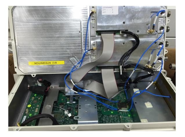
Photograph No.1 "AirHarmony 4000 700 MHz (B12/B17)" base station internal view
