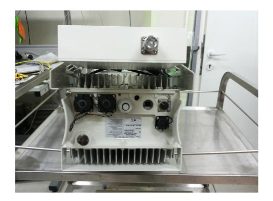
Photograph No.4 "AirHarmony 4000 700 MHz (B12/B17)" base station side view
