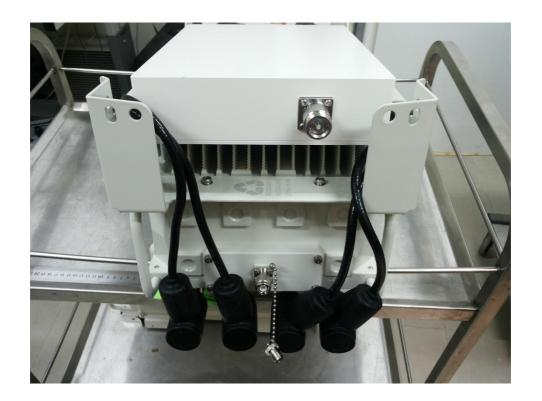
Photograph No.2 "AirHarmony 4000 700 MHz (B12/B17)" base station front side view
