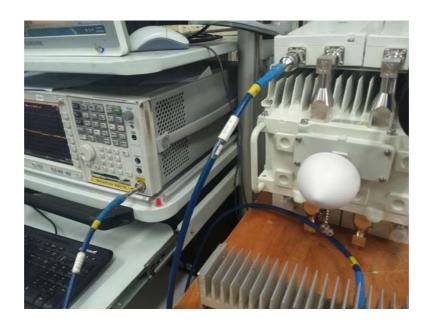
Photograph No.3 Occupied bandwidth measurement setup
