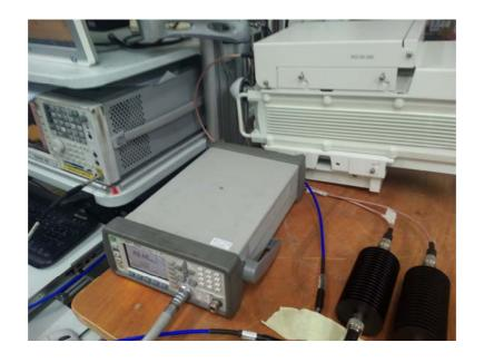
Photograph No.2 Conducted spurious and band edge emissions measurement setup
