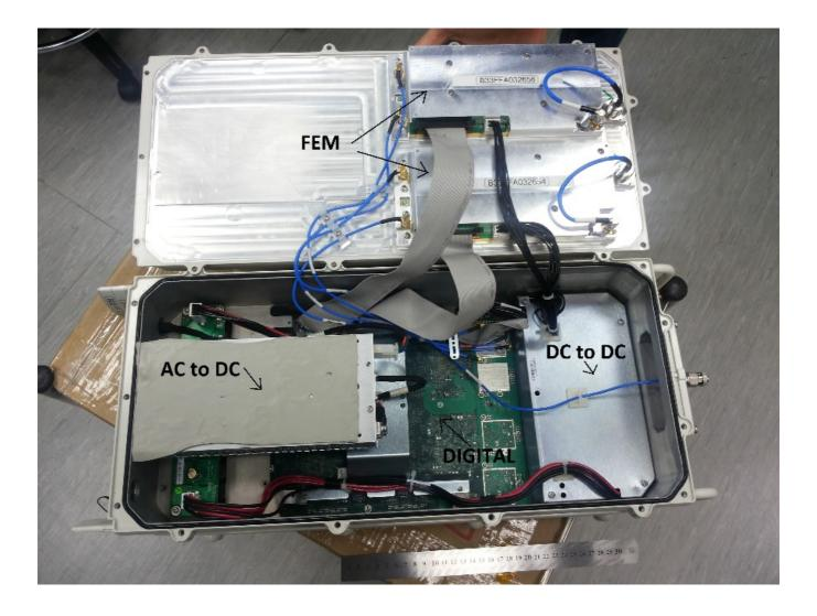
Photograph No.1 "AirHarmony 4400 2.5 GHz (B41)" base station internal view
