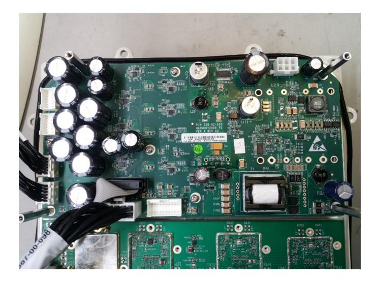
Photograph No.8 AC to DC power supply
