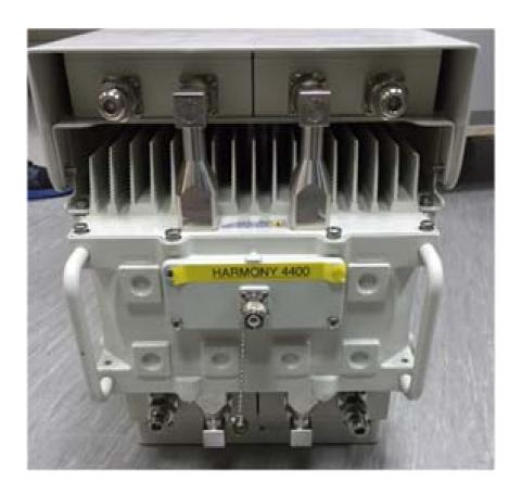
Photograph No.2 "AirHarmony 4400 2.5 GHz (B41)" base station bottom panel view
