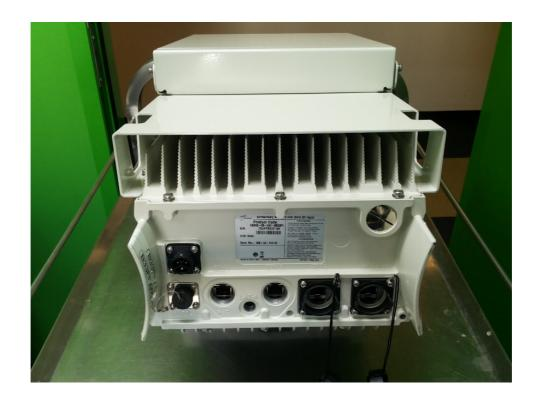
Photograph No.4 "AirHarmony 4000 2.5 GHz (B41)" base station side view
