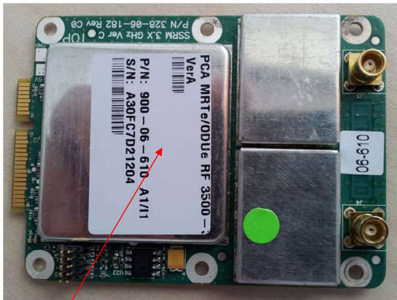
CRM 3.65GHz module, label with FCC ID:PIDCRM3650 location
