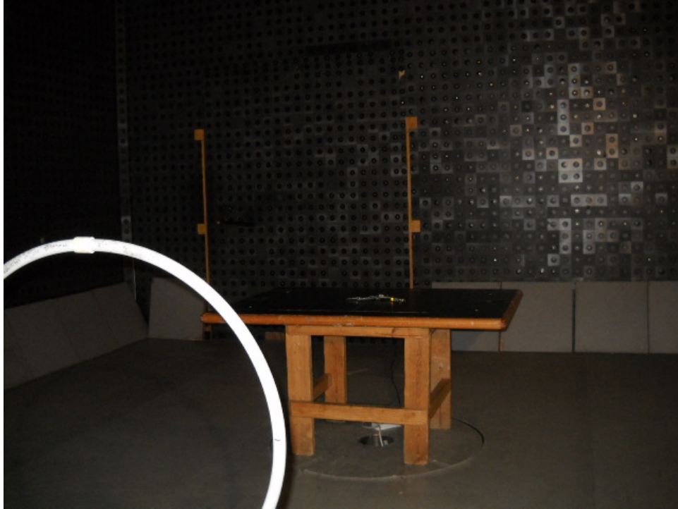
Photograph No.3 Spurious emissions measurement setup in the semi anechoic chamber below 30 MHz
