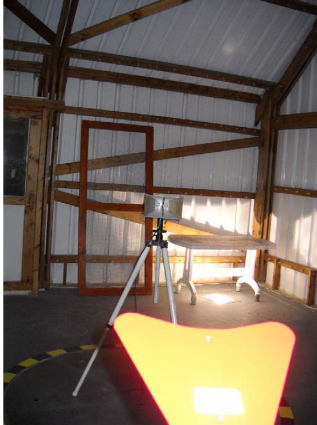
Photograph No.7 Substitution ERP measurement setup of spurious
