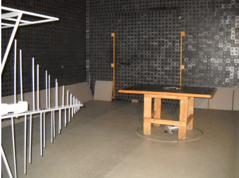
Photograph No.4 Spurious emissions measurement setup in the semi anechoic chamber in 30 -1000 MHz
