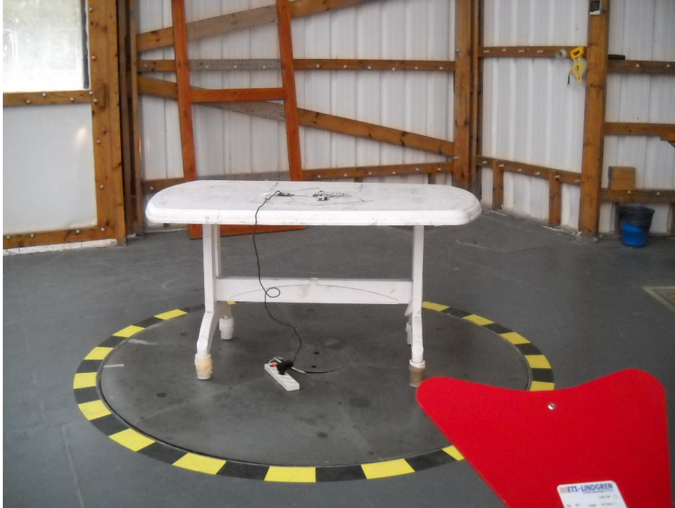
Photograph No.6 Spurious emissions measurement setup at OATS above 1000 MHz
