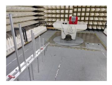
Photograph No.4 Spurious emissions measurement setup in the anechoic chamber above 18 GHz
