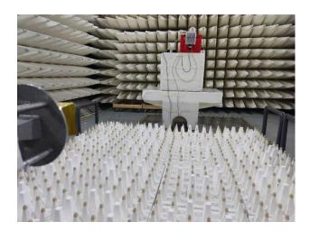
Photograph No.5 Frequency stability measurement setup
