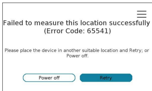
Figure 18 No signal detected
