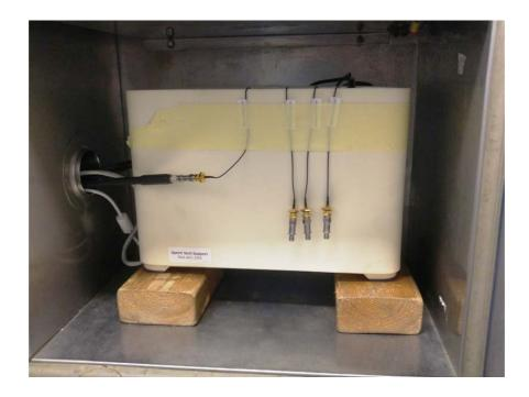
Photograph No.7 Frequency stability measurement setup
