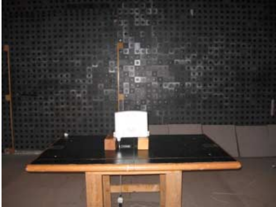
Photograph No.7 Spurious emissions measurement setup in the anechoic chamber, ProST close view
