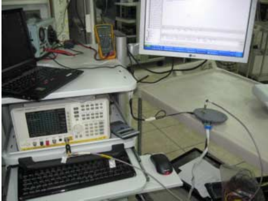
Photograph No.12 Frequency stability measurement setup
