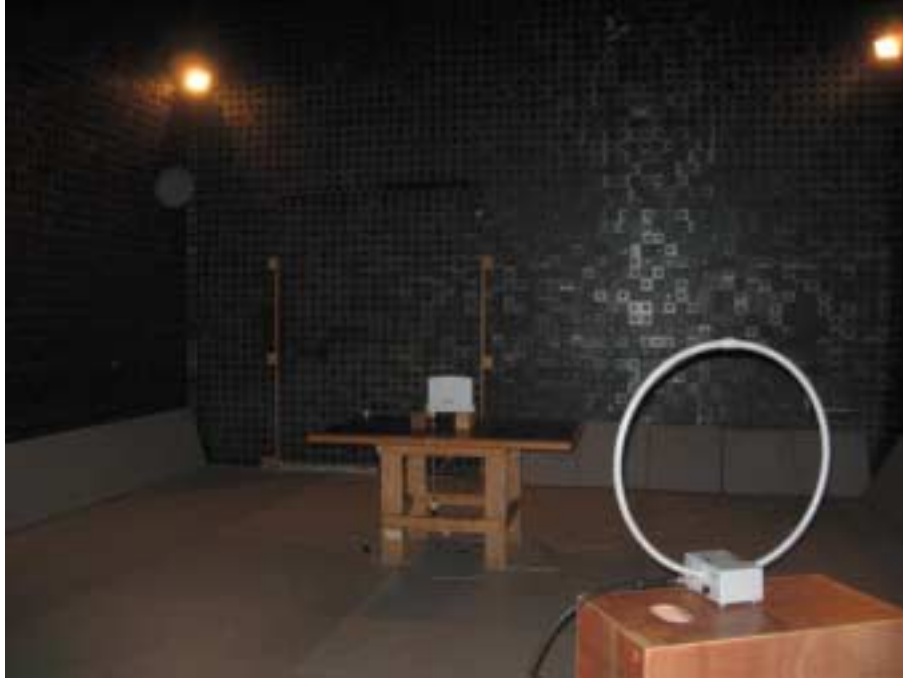
Photograph No.3 Spurious emissions measurement setup in the anechoic chamber below 30 MHz (ProST)
