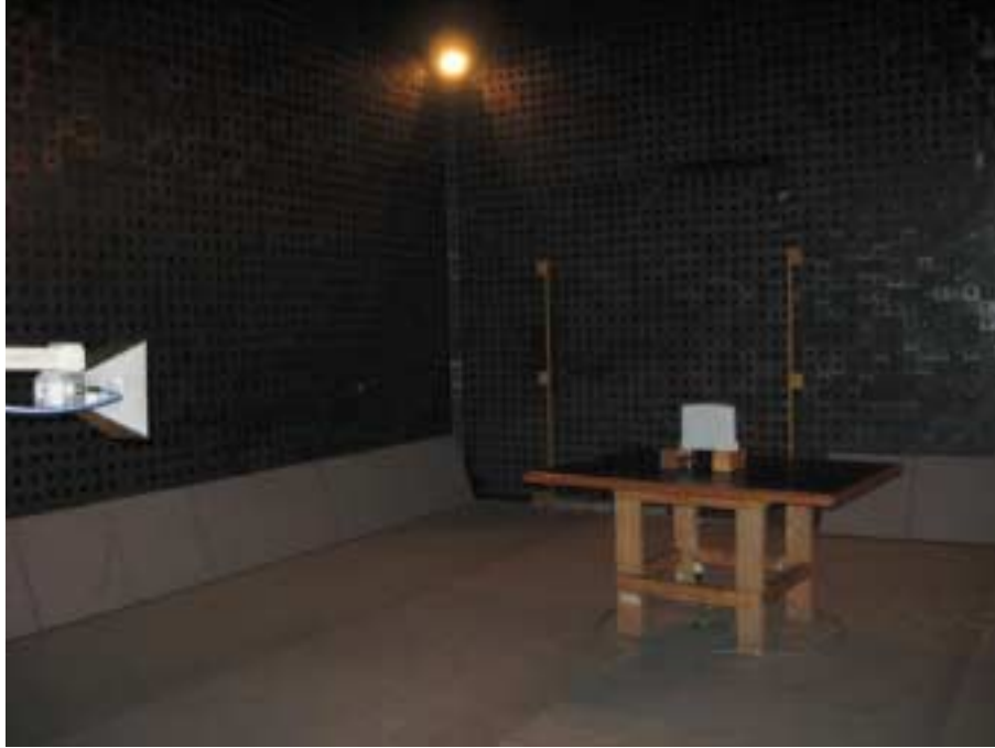
Photograph No.6 Radiated emissions measurement setup in the anechoic chamber above 1000 MHz (ProST)
