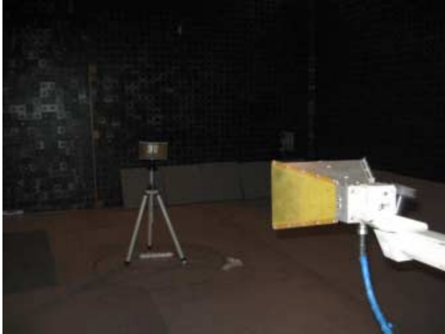
Photograph No.10 Setup of substitution ERP measurements of spurious in the anechoic chamber
