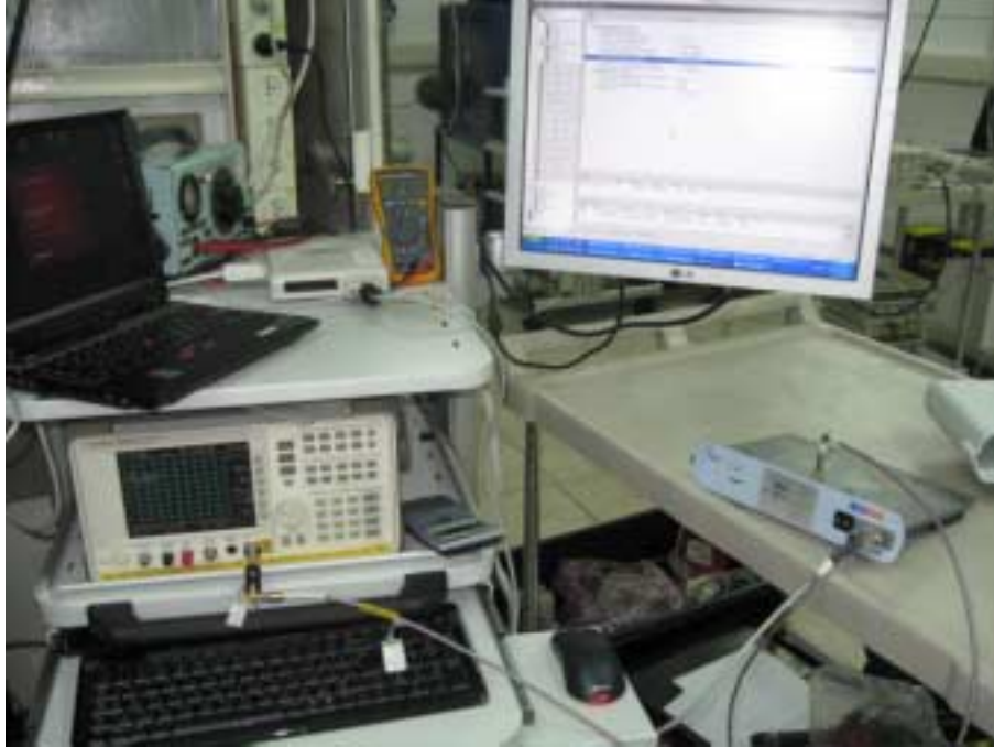
Photograph No.2 Occupied bandwidth, emission mask and conducted spurious emissions measurement setup
