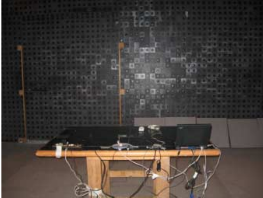
Photograph No.19 Radiated emissions measurement setup in the anechoic chamber (EasyST)
