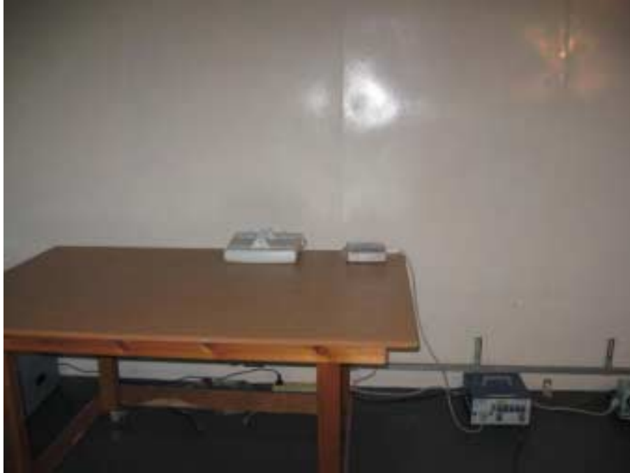
Photograph No.13 Conducted emissions measurement on AC line setup (ProST)
