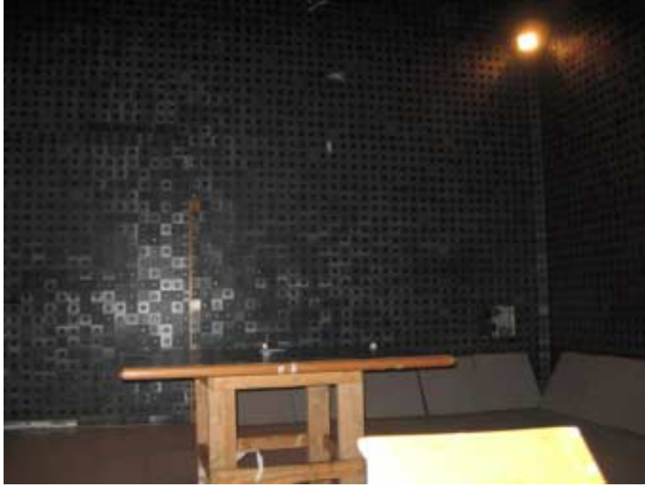
Photograph No.8 Radiated emissions measurement setup in the anechoic chamber above 1000 MHz (EasyST)
