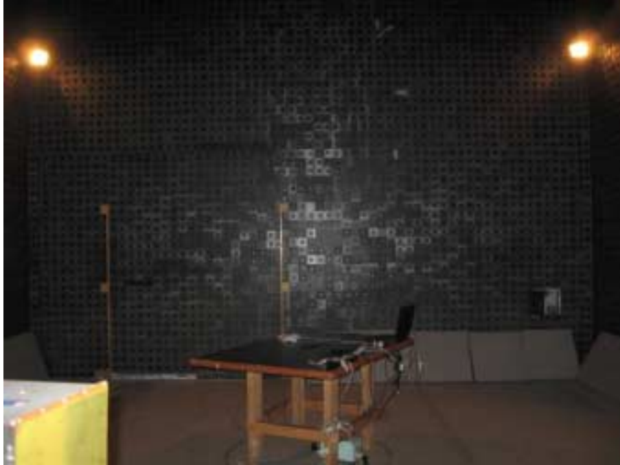
Photograph No.18 Radiated emissions measurement setup in the anechoic chamber (EasyST)
