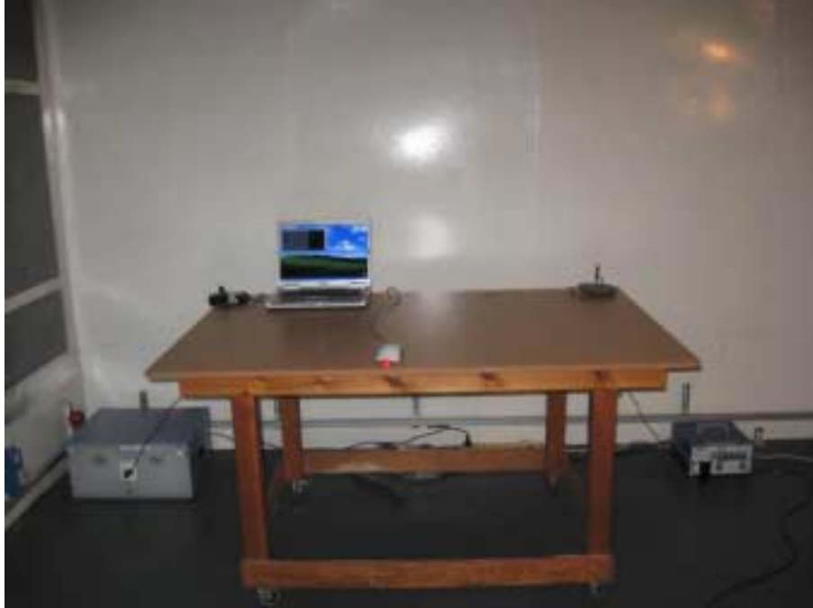
Photograph No.15 Conducted emissions measurement on AC line setup (EasyST)
