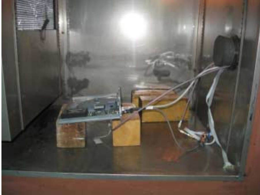
Photograph No.11 Frequency stability measurement setup
