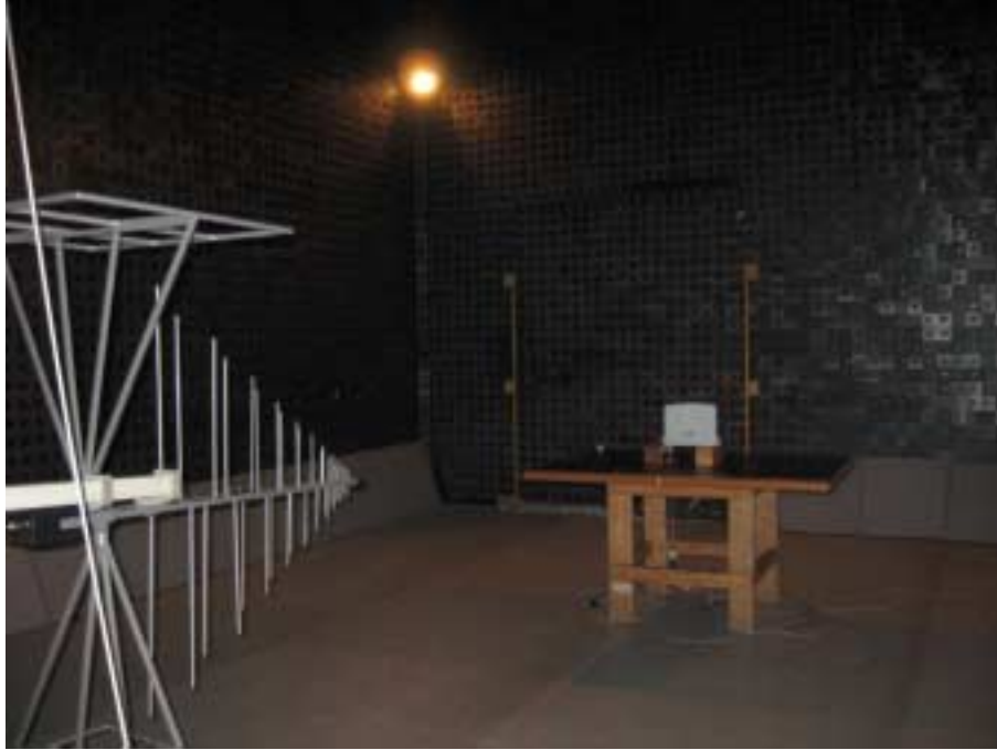
Photograph No.5 Spurious emissions measurement setup in the anechoic chamber in 30 -1000 MHz (ProST)
