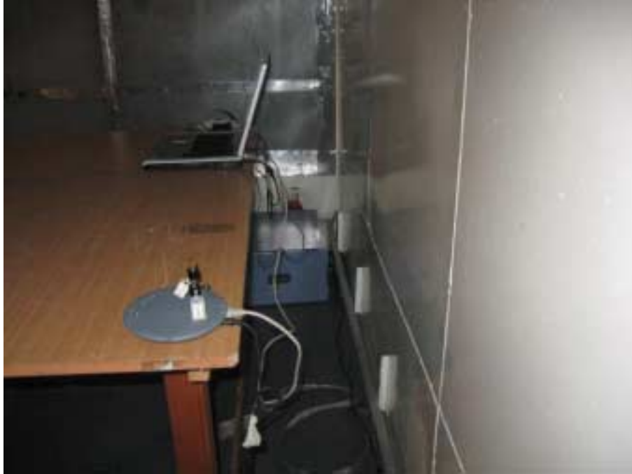
Photograph No.16 Conducted emissions measurement on AC line setup (EasyST)
