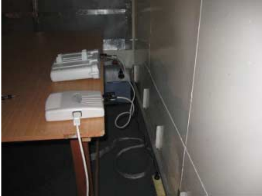
Photograph No.14 Conducted emissions measurement on AC line setup (ProST)
