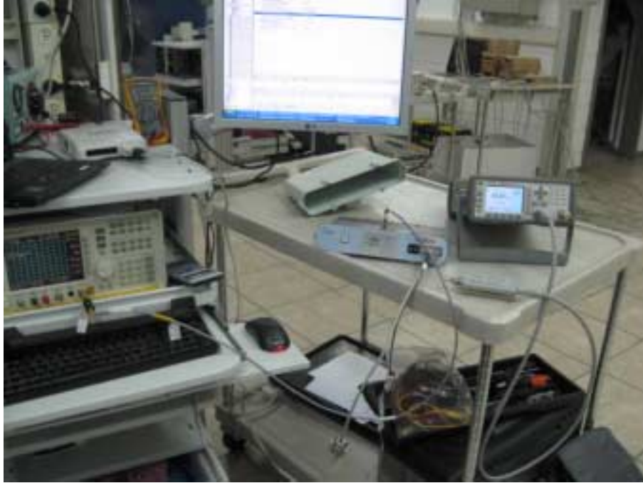
Photograph No.1 Peak output power measurement setup
