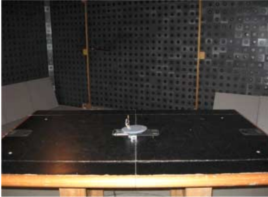
Photograph No.9 Spurious emissions measurement setup in the anechoic chamber, EasyST close view
