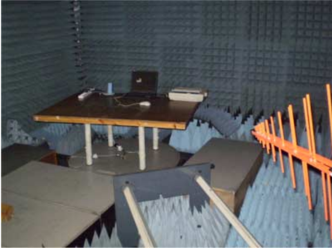
Photograph No.2 Spurious emissions measurement setup in the anechoic chamber in 30 – 1000 MHz
