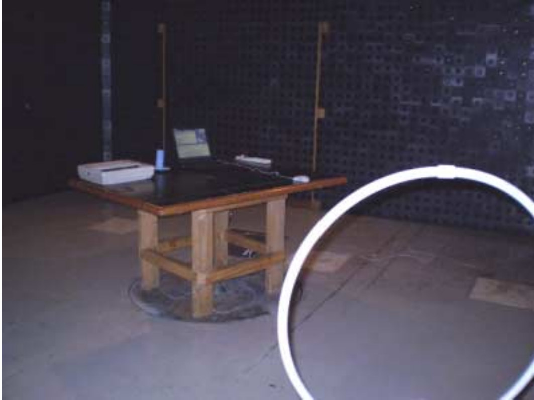
Photograph No.1 Spurious emissions measurement setup in the anechoic chamber below 30 MHz
