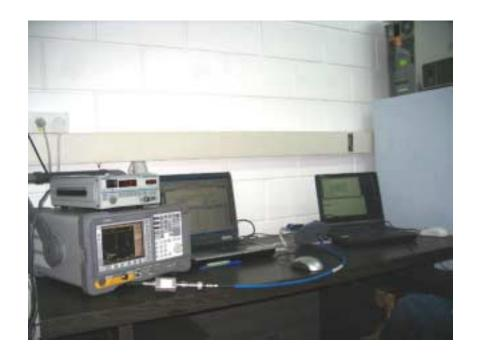
Photograph No.2 Occupied bandwidth, conducted spurious emissions measurement setup
