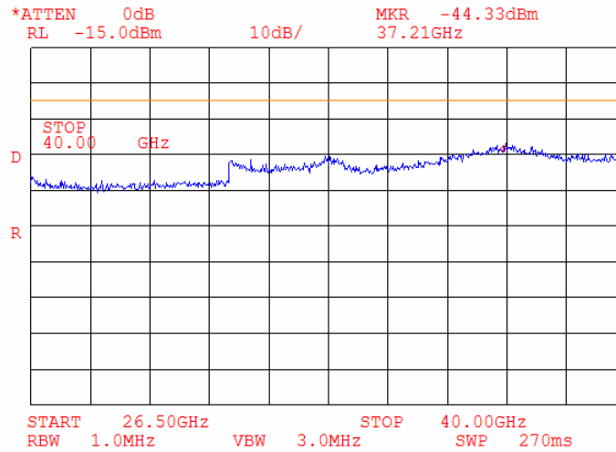
Plot 7.4.29 Spurious emission measurements in 26500 - 40000 MHz range at mid carrier frequency
