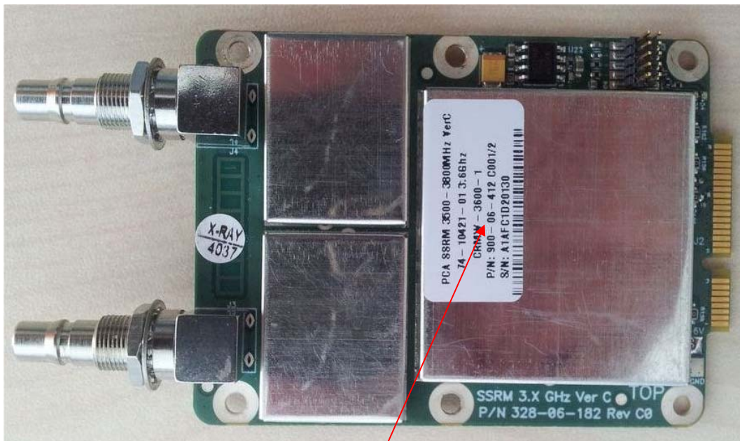
SSRM 3.65GHz module, label with FCC ID:PIDASMAX3700 location
