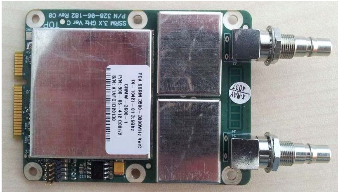
Photograph No.1 SSRM 3.65GHz module top view
