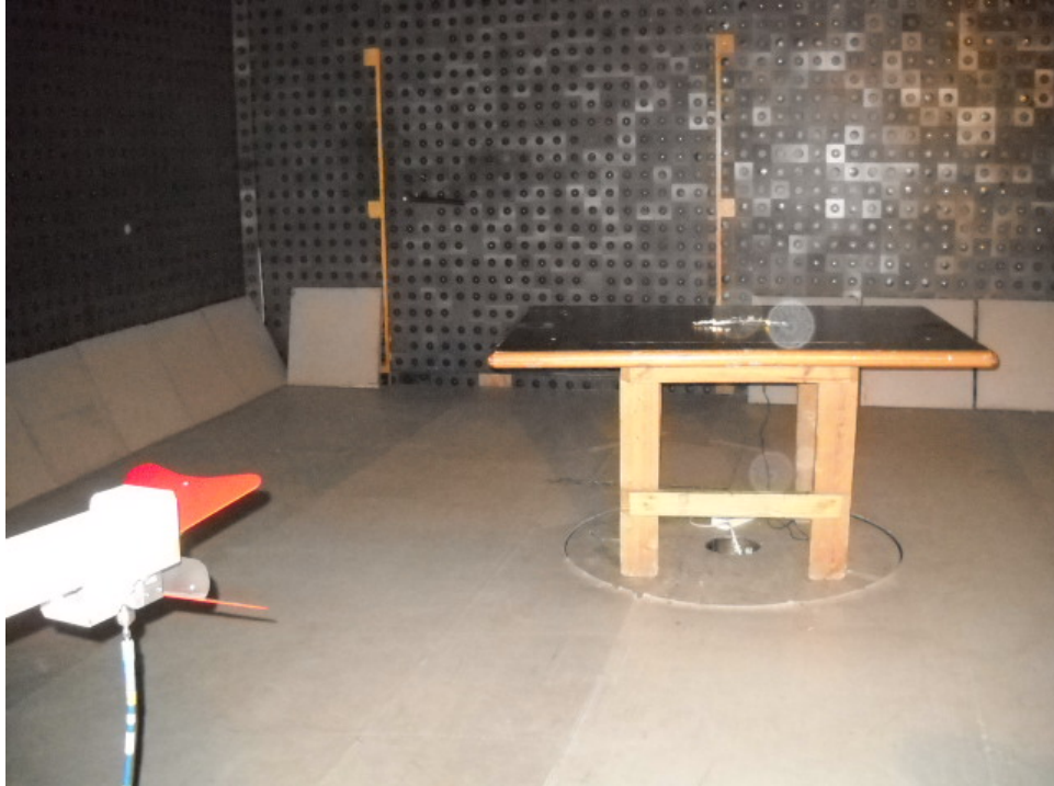
Photograph No.5 Spurious emissions measurement setup in the anechoic chamber above 1000 MHz
