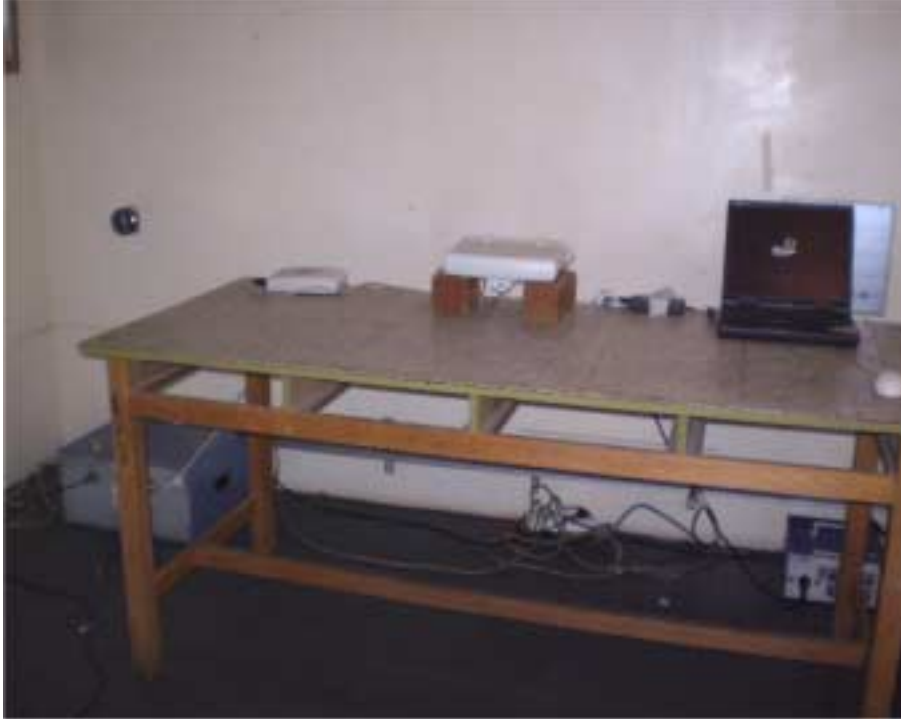
Photograph No.7 Conducted emissions measurement on AC line setup
