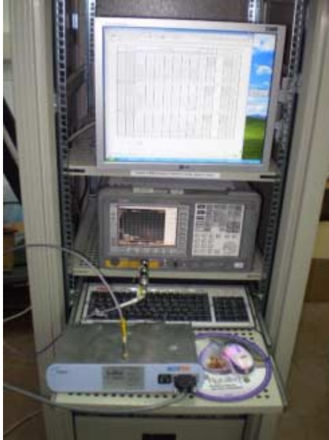
Photograph No.1 Peak output power, power spectral density, occupied bandwidth, conducted spurious emissions measurement setup
