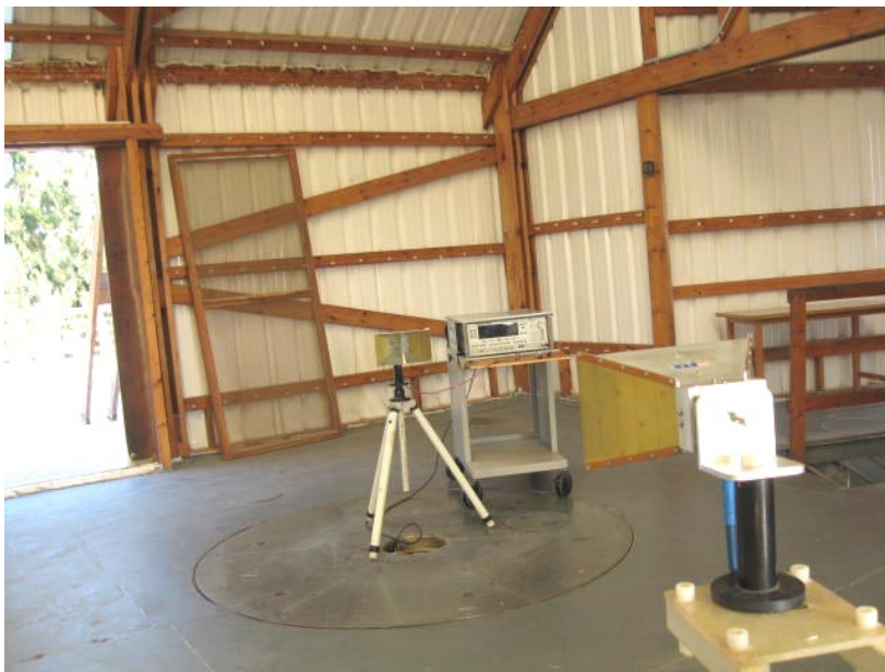
Photograph No.6 Setup for substitution method of spurious ERP measurements
