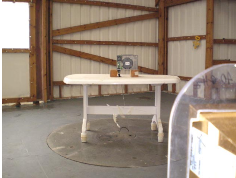
Photograph No.5 Spurious emissions measurement setup at the OATS above 1000 MHz
