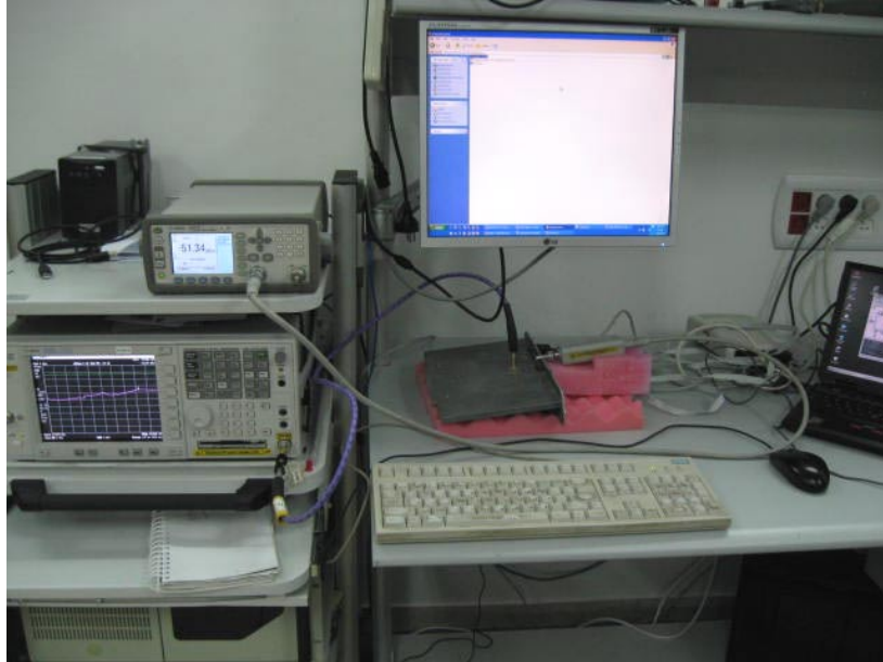
Photograph No.1 Peak output power, occupied bandwidth, emission mask, conducted spurious emissions measurement setup
