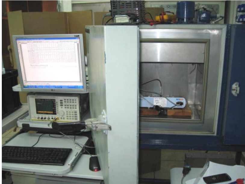
Photograph No.7 Frequency stability measurement setup
