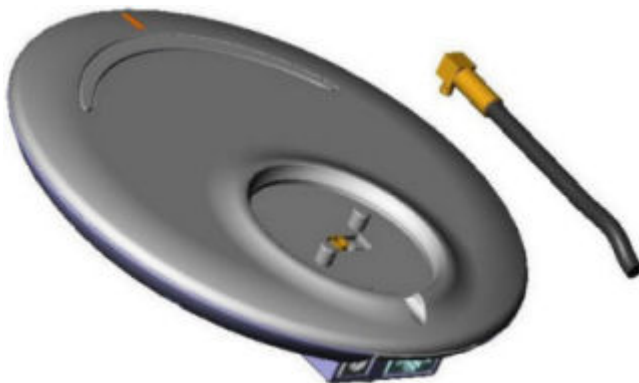
Figure 26 - Unplug MCX connector
