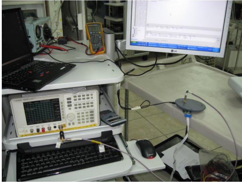
Photograph No.5 Frequency stability measurement setup
