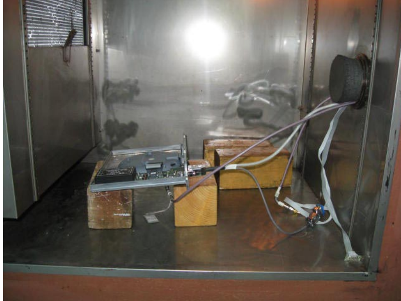
Photograph No.6 Frequency stability measurement setup
