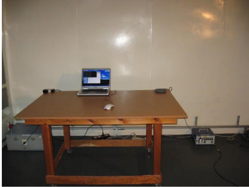
Photograph No.7 Conducted emissions measurement on AC line setup
