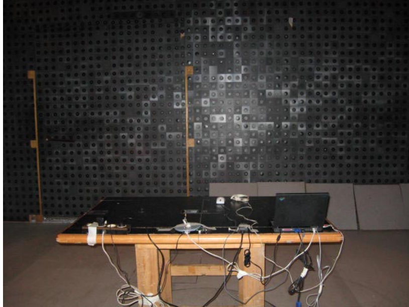
Photograph No.10 Radiated emissions measurement setup in the anechoic chamber, close view
