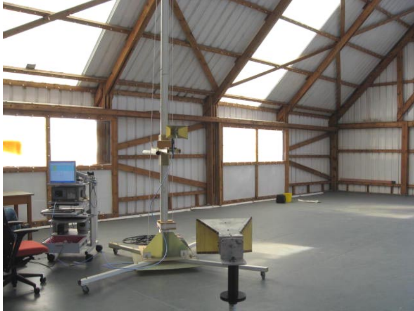
Photograph No.4 Setup of substitution ERP measurements of spurious at the OATS
