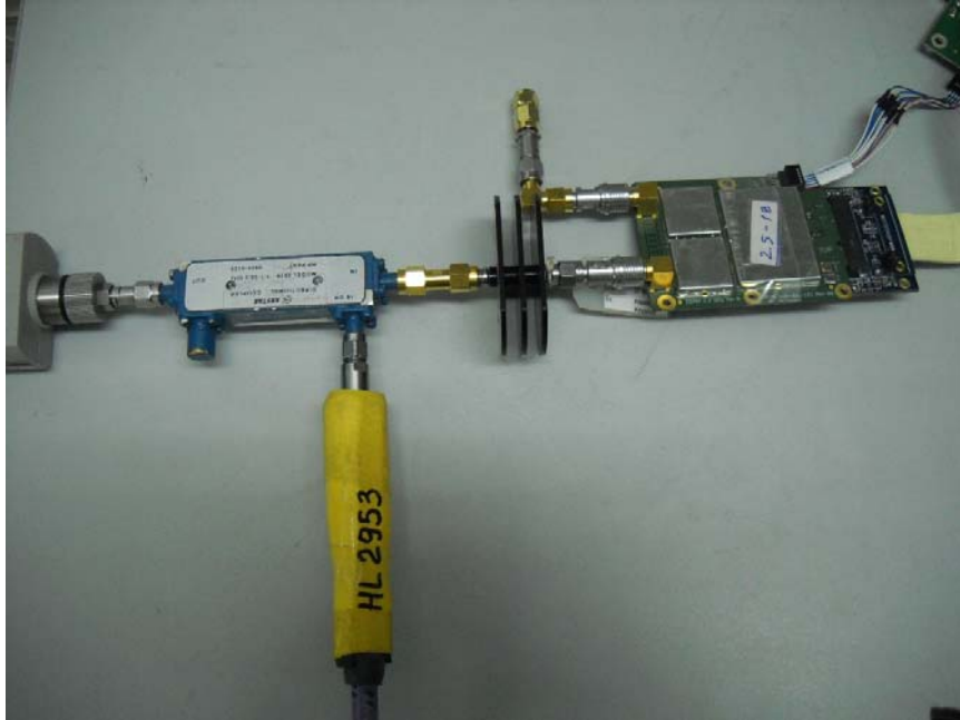
Photograph No.2 Occupied bandwidth measurement setup
