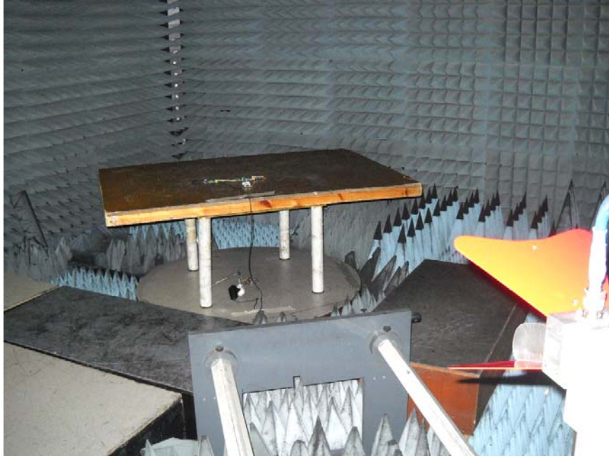
Photograph No.5 Spurious emissions measurement setup in the anechoic chamber above 1 GHz
