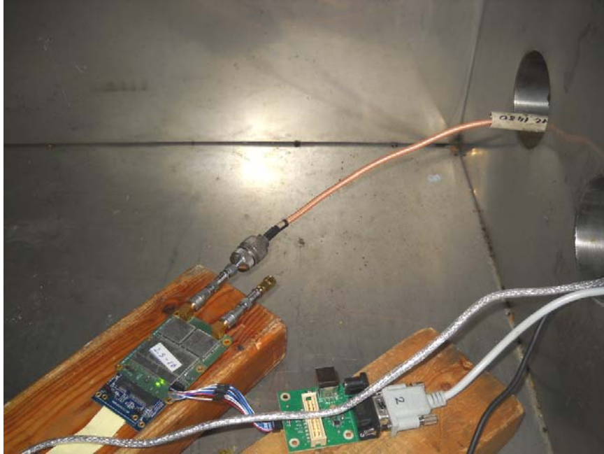
Photograph No.9 Frequency stability measurement setup
