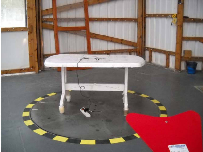
Photograph No.6 Spurious emissions measurement setup at the OATS in 1 – 18 GHz
