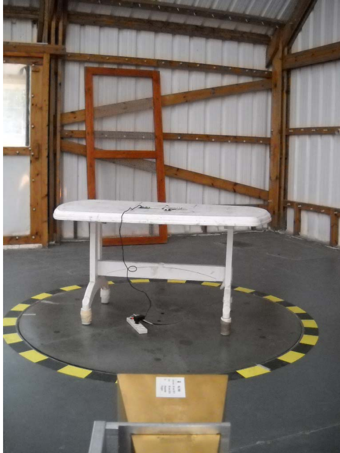
Photograph No.7 Spurious emissions measurement setup at the OATS in 18 – 27 GHz
