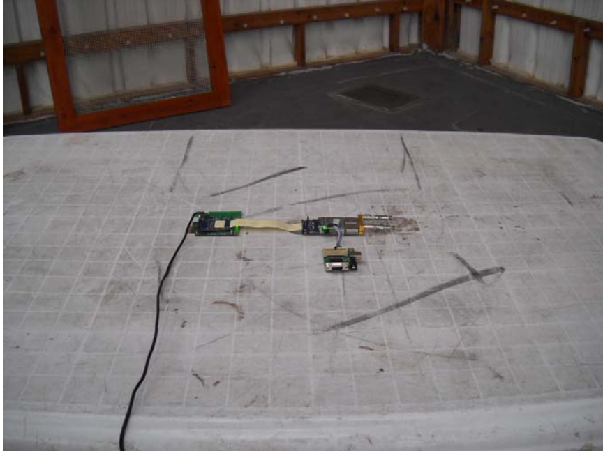
Photograph No.8 Radiated emissions measurement setup at the OATS, EUT close view
