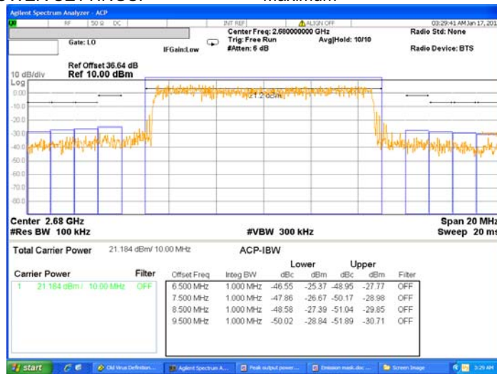
Plot 7.3.22 Emission mask test results at low carrier frequency, 10 MHz EBW
