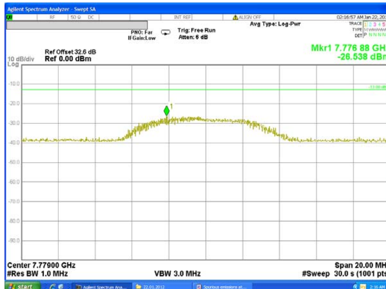
Plot 7.5.17 Conducted spurious emission measurements at the 3 rd harmonic of mid carrier frequency
