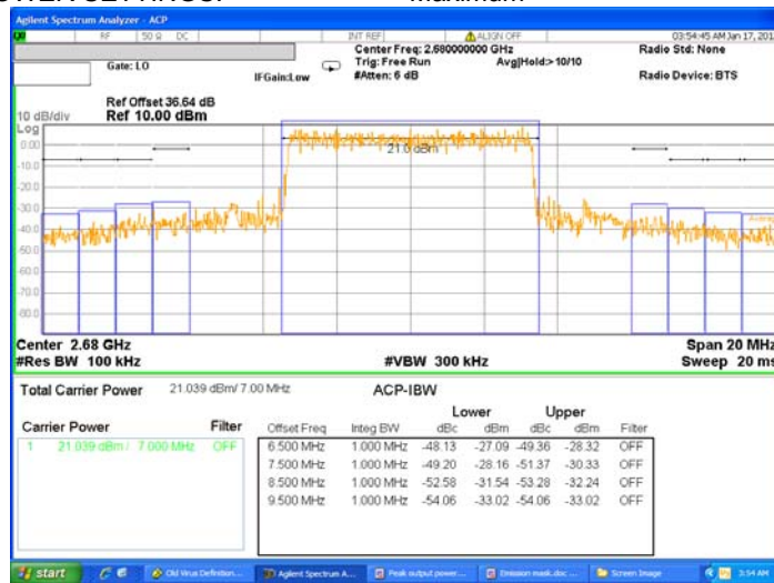
Plot 7.3.16 Emission mask test results at low carrier frequency, 7 MHz EBW
