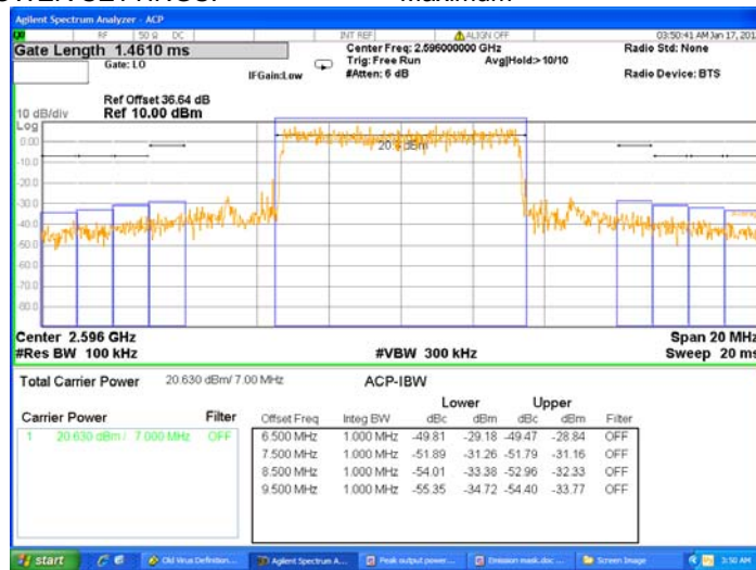
Plot 7.3.18 Emission mask test results at high carrier frequency, 10 MHz EBW
