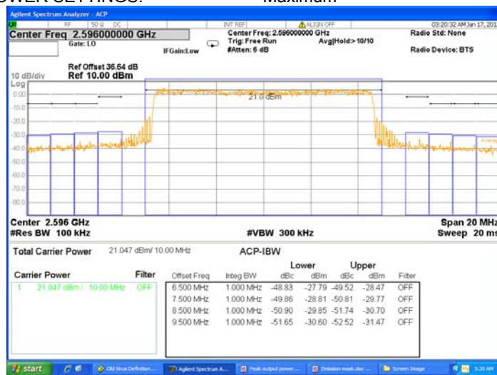
Plot 7.3.24 Emission mask test results at high carrier frequency, 10 MHz EBW
