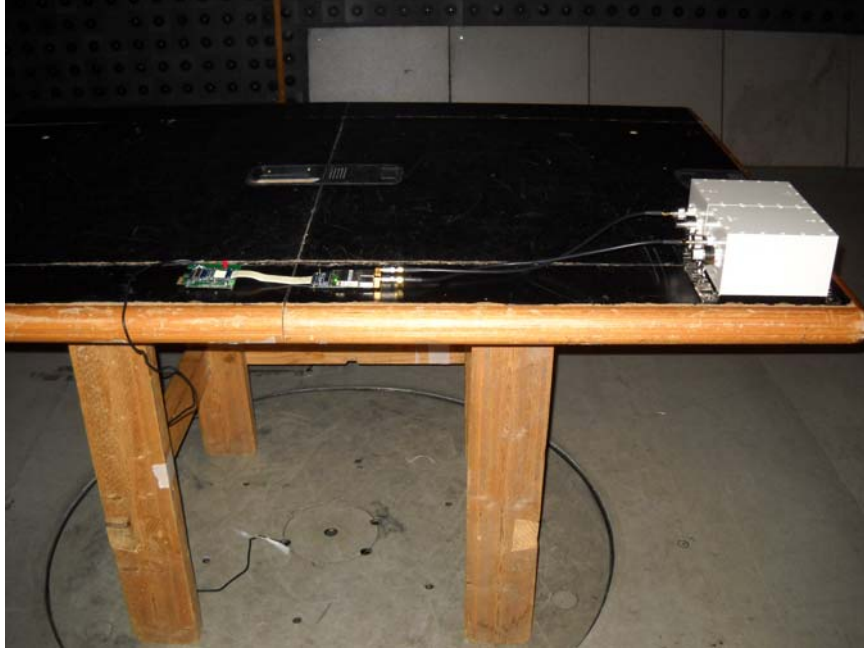
Photograph No.6 Radiated emissions measurement setup in the anechoic chamber, EUT close view
