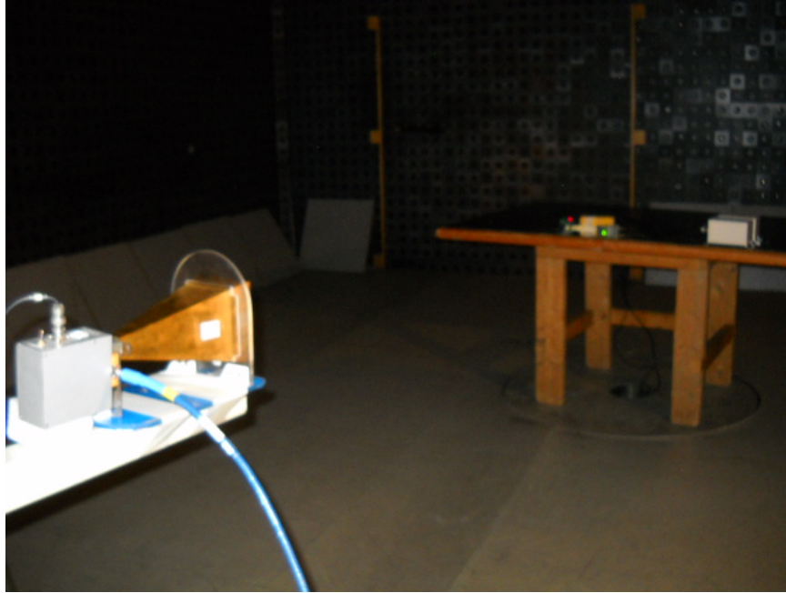
Photograph No.5 Spurious emissions measurement setup in the anechoic chamber in 18-24 GHz range
