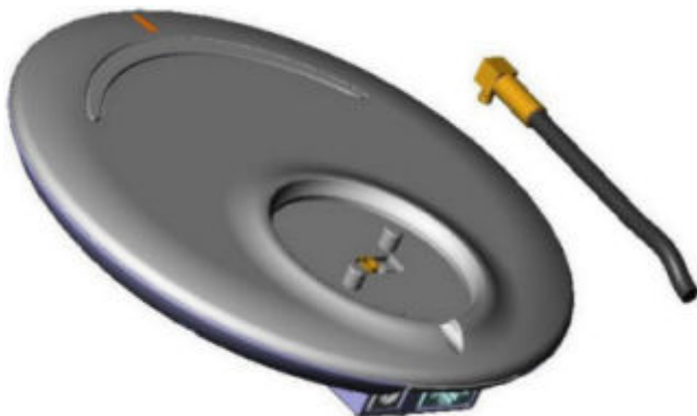
Figure 26 - Unplug MCX connector
