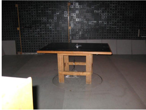
Photograph No.8 Spurious emissions measurement setup in the anechoic chamber above 1000 MHz (EasyST)
