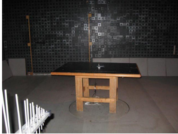
Photograph No.7 Spurious emissions measurement setup in the anechoic chamber in 30 -1000 MHz (EasyST)
