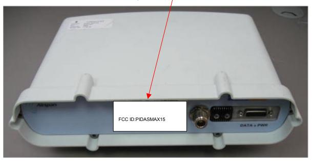
"EasyST 1.4G TDD" bottom panel, label with FCC ID:PIDASMAX15 location
