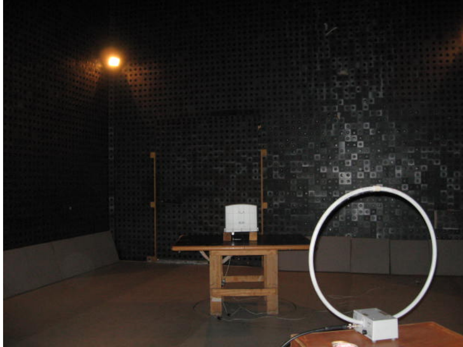
Photograph No.3 Spurious emissions measurement setup in the anechoic chamber below 30 MHz
