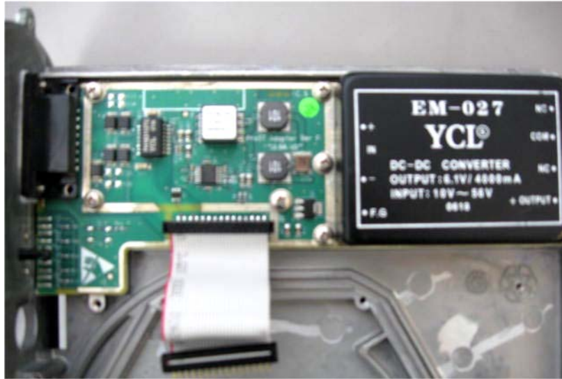
Photograph No.2 “ProST 1.4G TDD V-p” power supply close view
