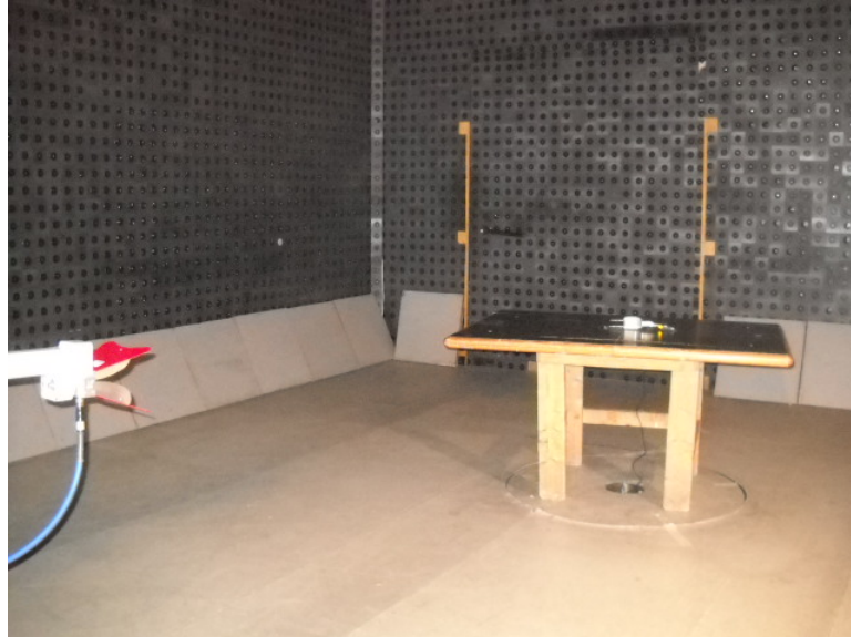
Photograph No.7 Spurious emissions measurement setup in the anechoic chamber above 1 GHz
