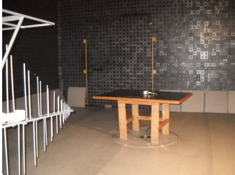
Photograph No.6 Spurious emissions measurement setup in the anechoic chamber in 30 -1000 MHz
