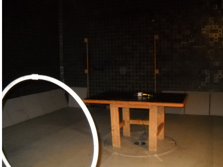
Photograph No.5 Spurious emissions measurement setup in the anechoic chamber below 30 MHz
