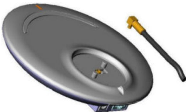
Figure 26 - Unplug MCX connector
