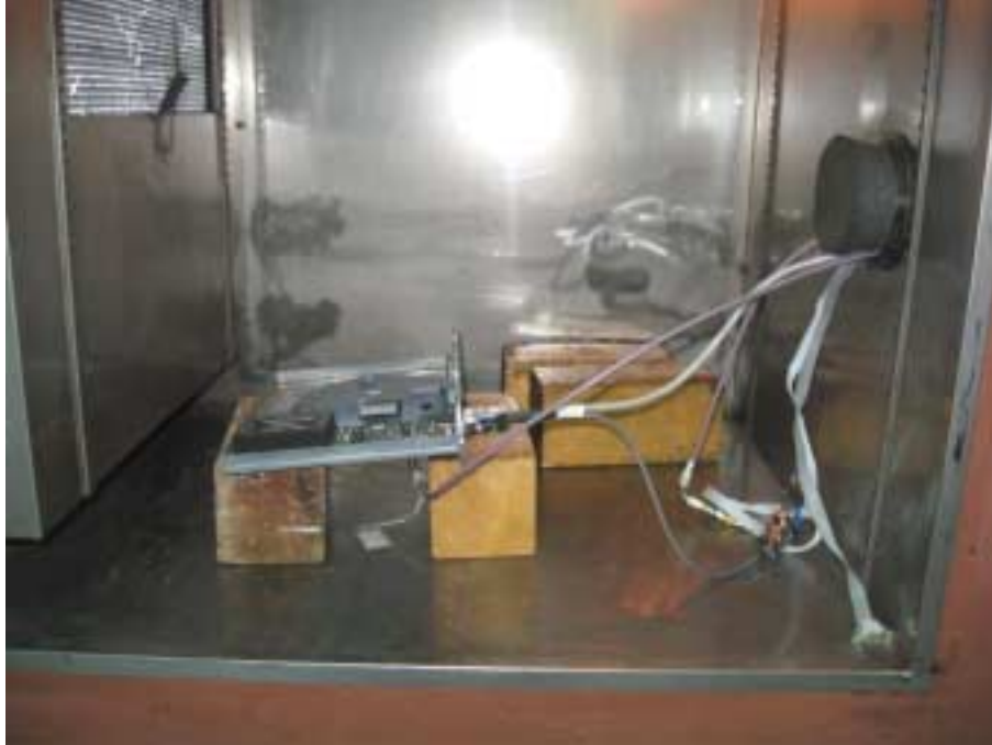
Photograph No.9 Frequency stability measurement setup
