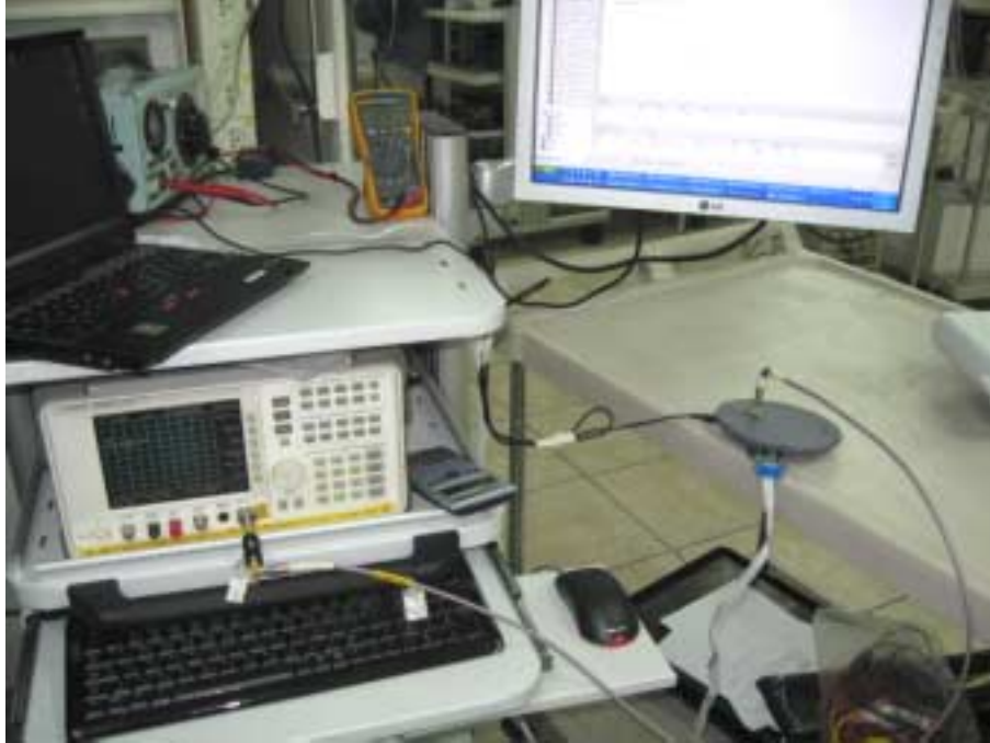
Photograph No.10 Frequency stability measurement setup (EasyST)
