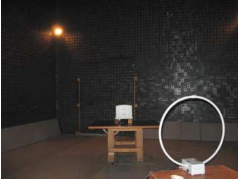
Photograph No.2 Spurious emissions measurement setup in the anechoic chamber below 30 MHz (ProST)
