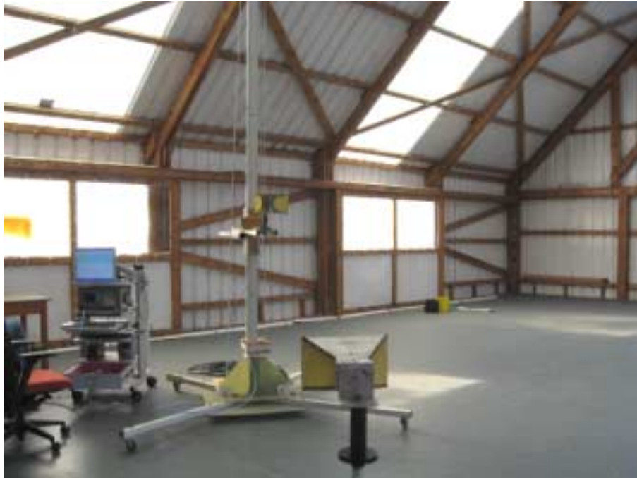
Photograph No.8 Setup of substitution ERP measurements of spurious at the OATS
