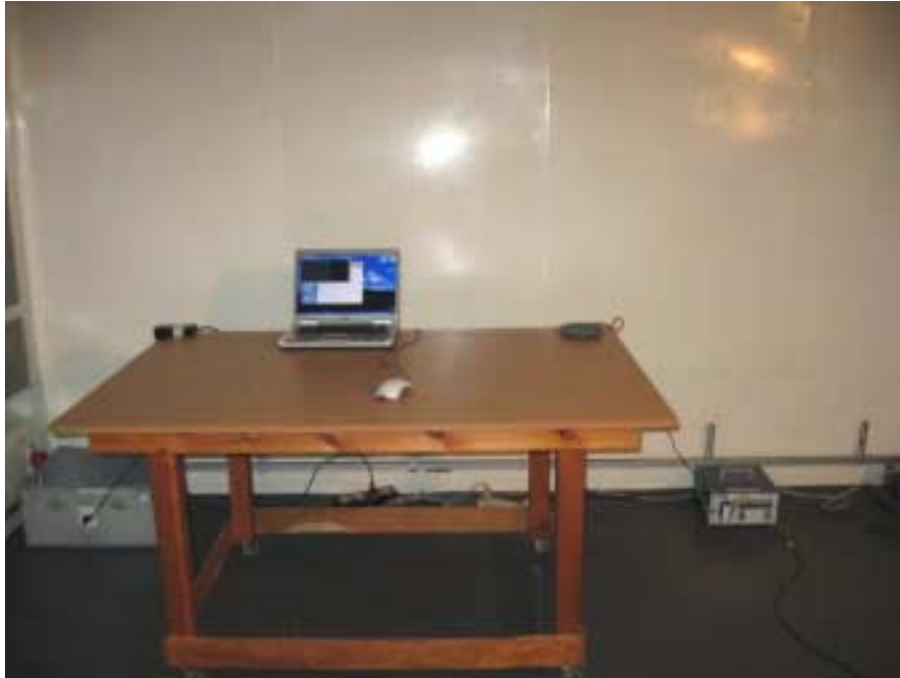
Photograph No.13 Conducted emissions measurement on AC line setup (EasyST)
