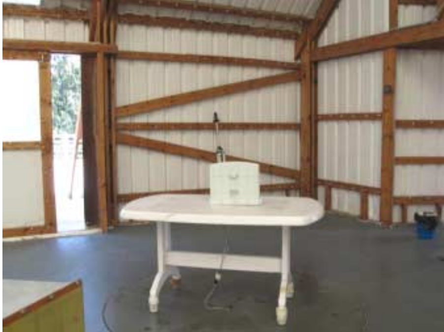
Photograph No.7 Radiated emissions measurement setup at the OATS above 1000 MHz (ProST)
