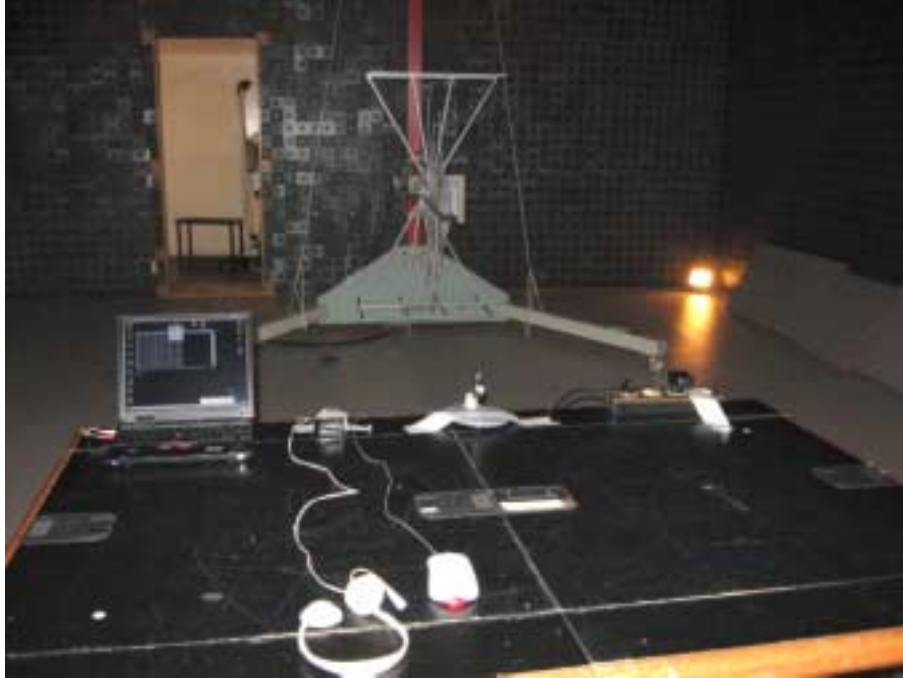
Photograph No.15 Radiated emissions measurement setup in the anechoic chamber (EasyST)
