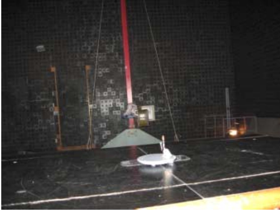
Photograph No.6 Spurious emissions measurement setup in the anechoic chamber above 1000 MHz (EasyST)
