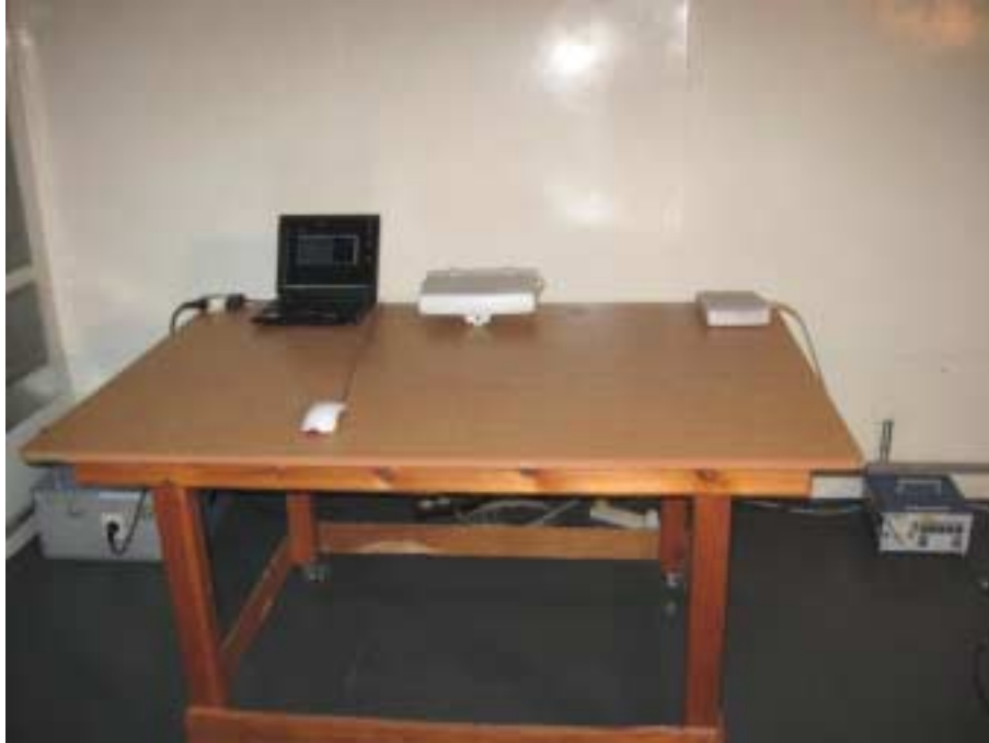
Photograph No.11 Conducted emissions measurement on AC line setup (ProST)
