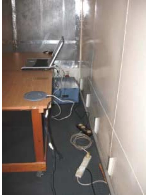
Photograph No.14 Conducted emissions measurement on AC line setup (EasyST)
