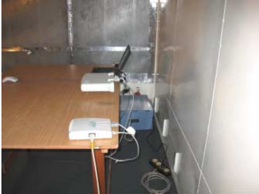
Photograph No.12 Conducted emissions measurement on AC line setup (ProST)
