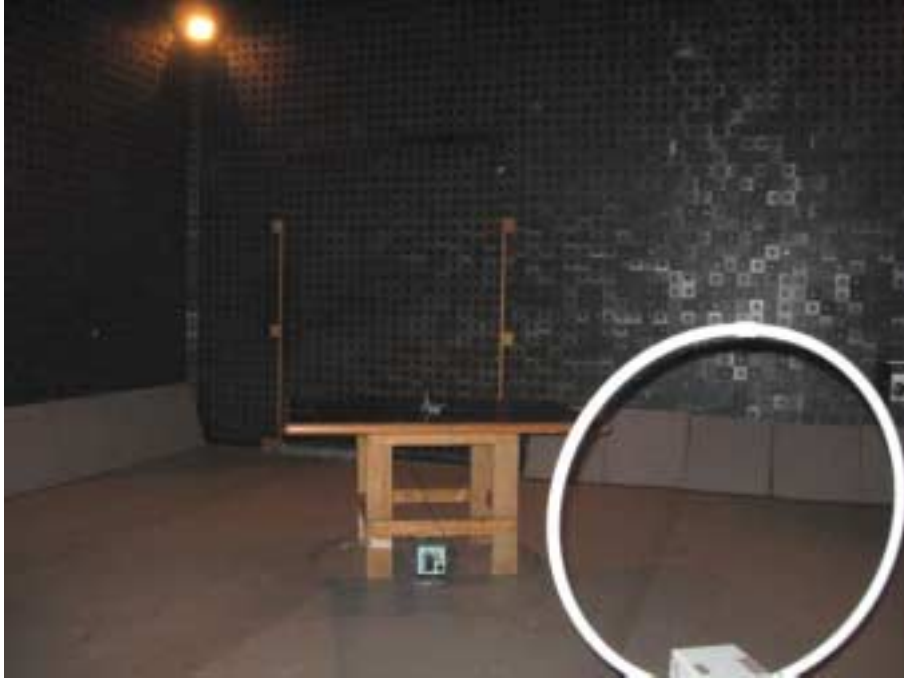
Photograph No.3 Spurious emissions measurement setup in the anechoic chamber below 30 MHz (EasyST)
