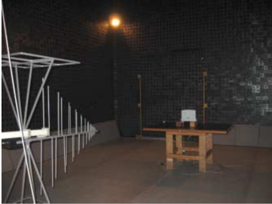
Photograph No.4 Spurious emissions measurement setup in the anechoic chamber in 30 -1000 MHz (ProST)
