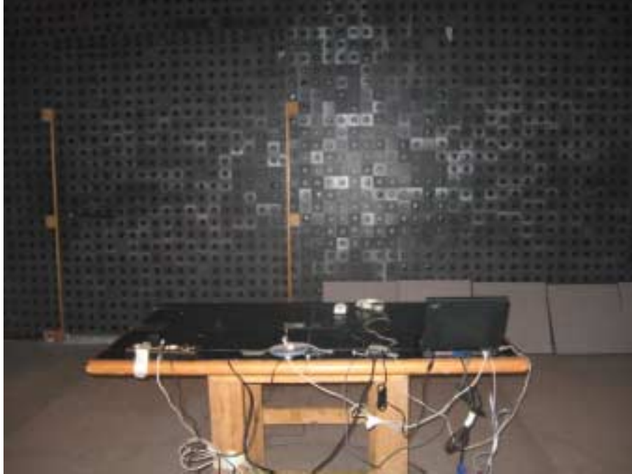
Photograph No.17 Radiated emissions measurement setup in the anechoic chamber (EasyST)
