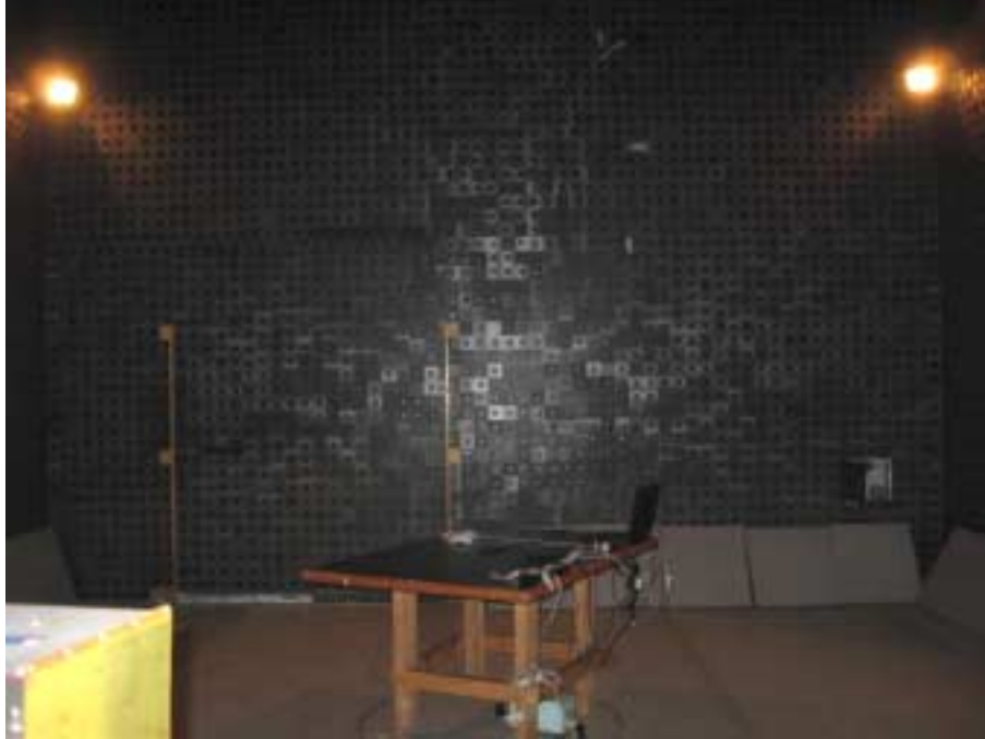
Photograph No.16 Radiated emissions measurement setup in the anechoic chamber (EasyST)
