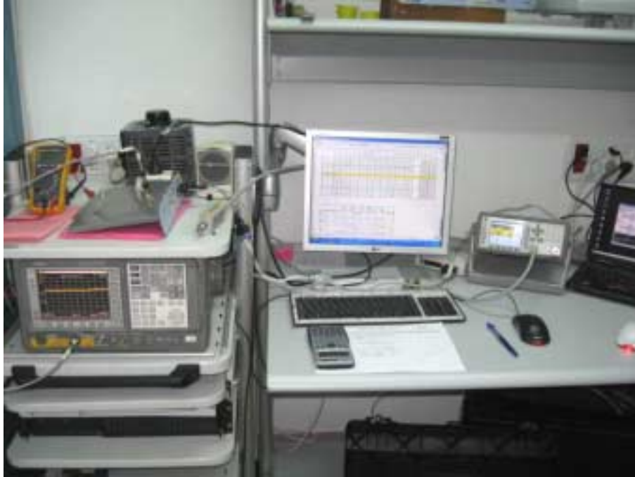
Photograph No.1 Peak output power, occupied bandwidth and conducted spurious emissions measurement setup
