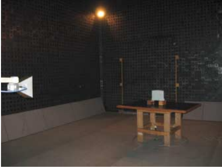
Photograph No.5 Spurious emissions measurement setup in the anechoic chamber above 1000 MHz (ProST)
