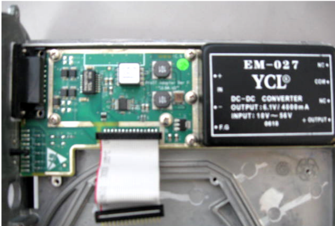
Photograph No.2 "ProST 1.4G TDD" power supply close view
