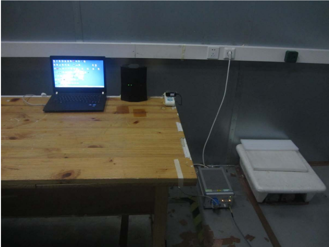
Picture 3 Conducted Emission Test Setup
