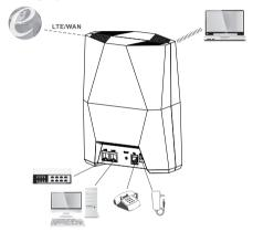
Step 1 Connect the supplied power adapter to the CPE. Step 2 Connect other devices.
