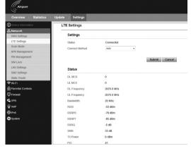
The default configuration are Auto connect and Scan full band. If you want to connect to the 4G network according to your requirements, set the Connect Method to Manual, and scan a specified band.
