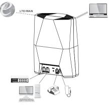
Step 1 Connect the supplied power adapter to the CPE. Step 2 Connect other devices.
