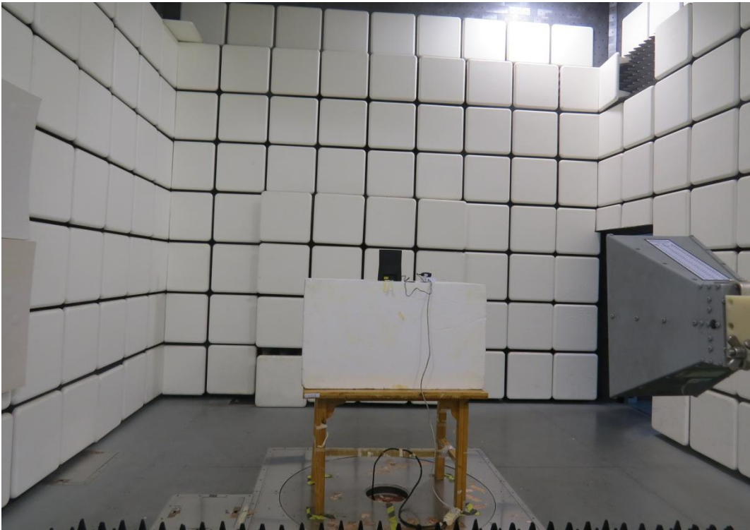
Picture 2 Radiated Spurious Emissions Test setup
