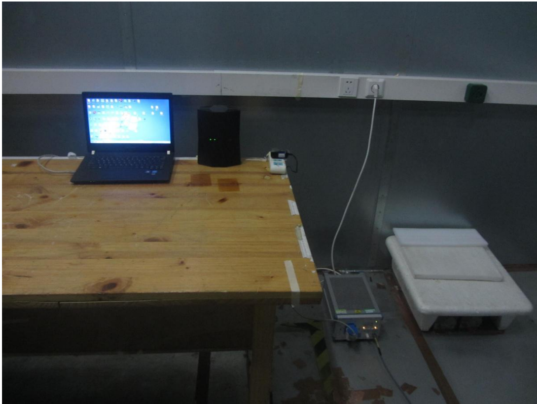
Picture 3 Conducted Emission Test Setup
