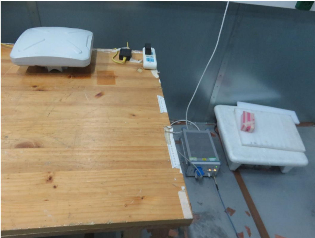
Picture 3 Radiated Emission Test Setup
